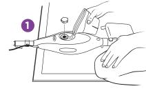
1 Turn the water tank cap counter clockwise and remove from the tank.
